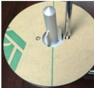
Frame installation: remove the two hexagon socket screws at the back of the machine, fix the frame as shown in the picture and lock the screws
