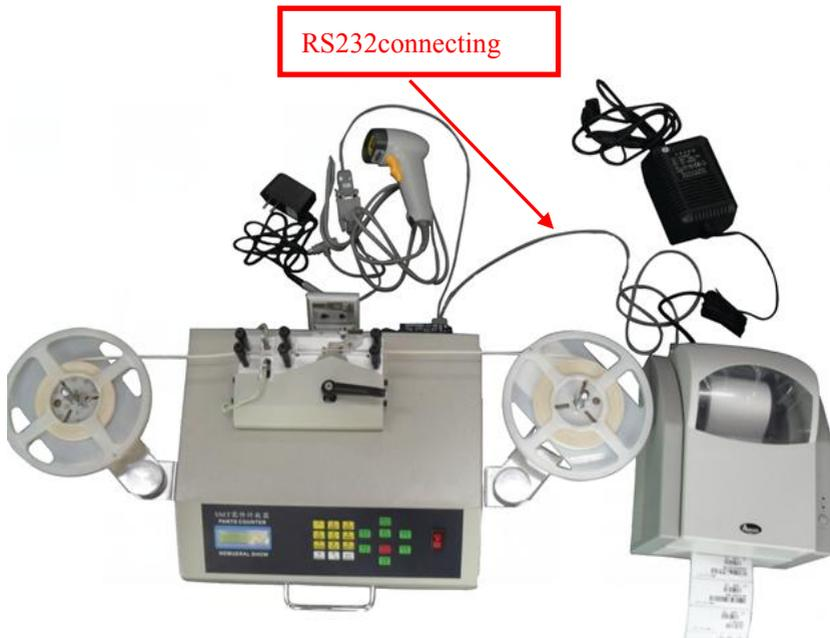
**Note: there will be a two-part RS232 connection line in the accessories of the printer and scanning gun, the female head will be connected to the rear interface of the machine, the two male heads will be connected, the long line will be connected to the printer, and the short line will be connected to the scanning gun**
